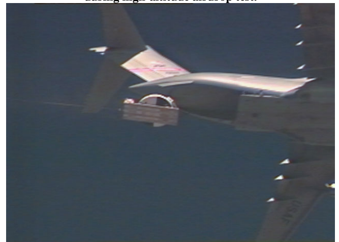
Figure 1 – Drogue extraction of Orion CPAS from the C-17A during high-altitude airdrop test.
