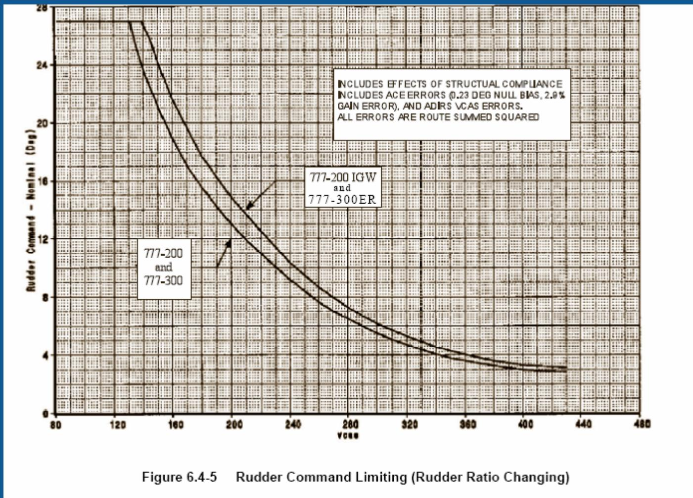
Figure 6.4-5 Rudder Command Limiting (Rudder Ratio Changing)
