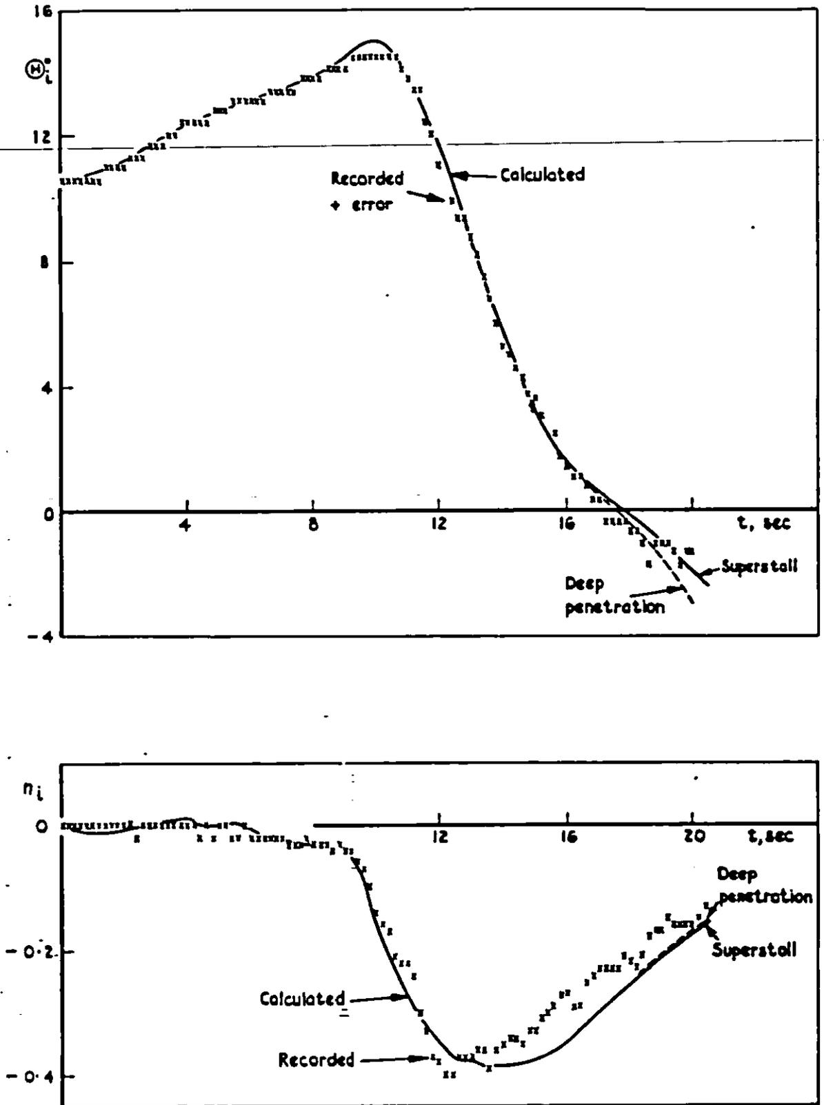
Fig.1 Pitch attitude (angle of inclination),  $H_i$ , and indicated normal acceleration factor
