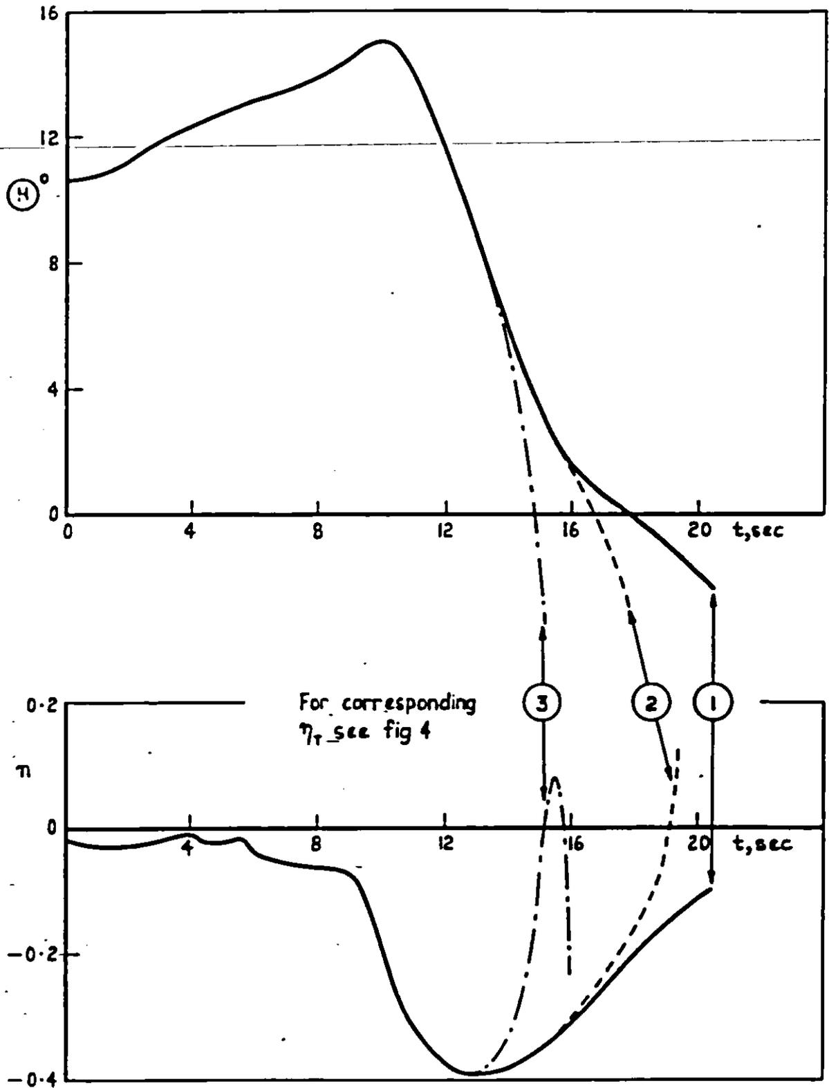
Fig. 5 Effect of different recovery action on pitch attitude (angle of inclination),  $\textcircled{H}$  and on normal acceleration factor,  $n$
