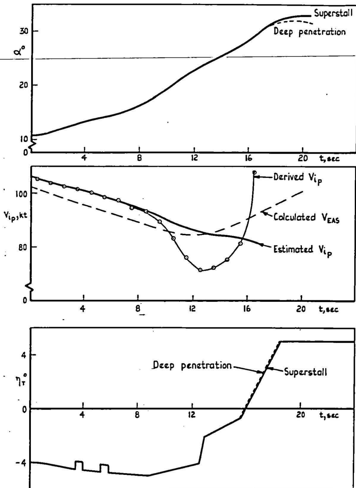
Fig. 3 Angle of incidence,  $\alpha$ , velocity indicated to pilot,  $V_{ip}$  and tailplane angle,  $\eta_r$
