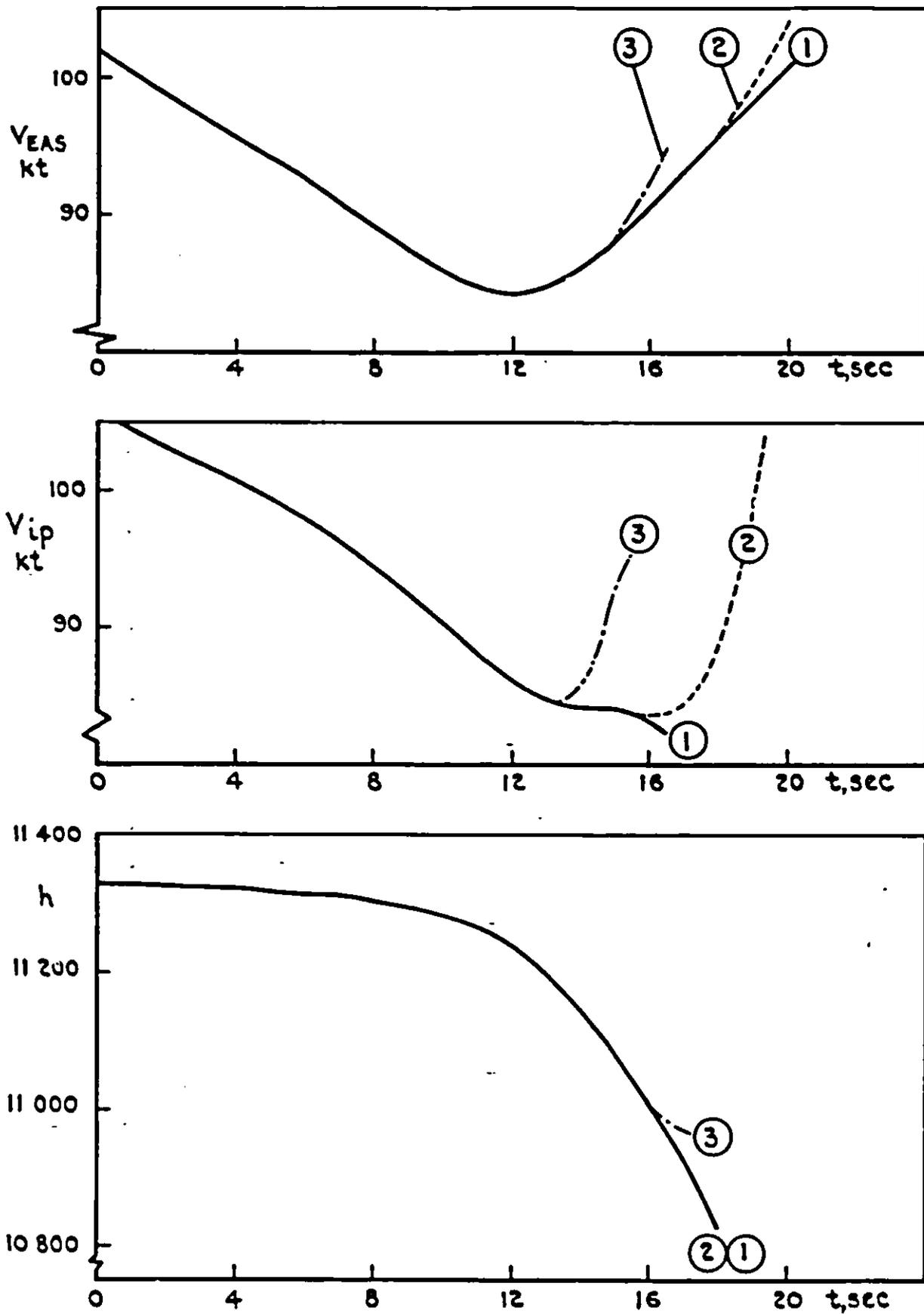
Fig. 6 Effect of different recovery action on airspeed (EAS & IAS) and height
