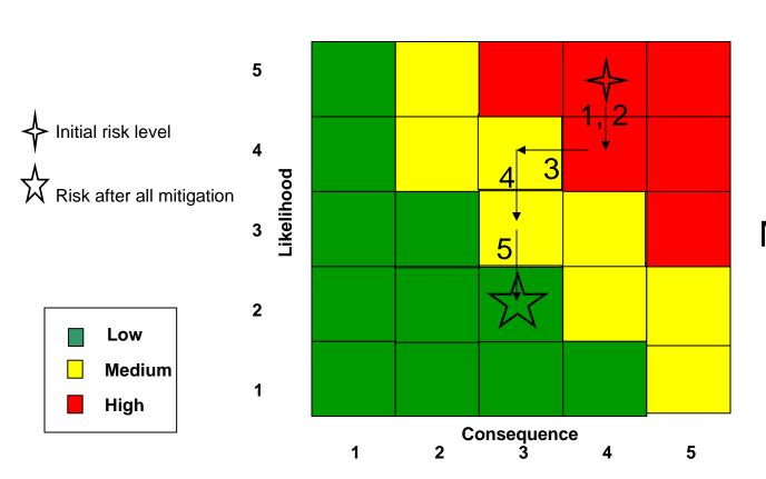
Mitigations lower likelihood & consequence of new component failures.
