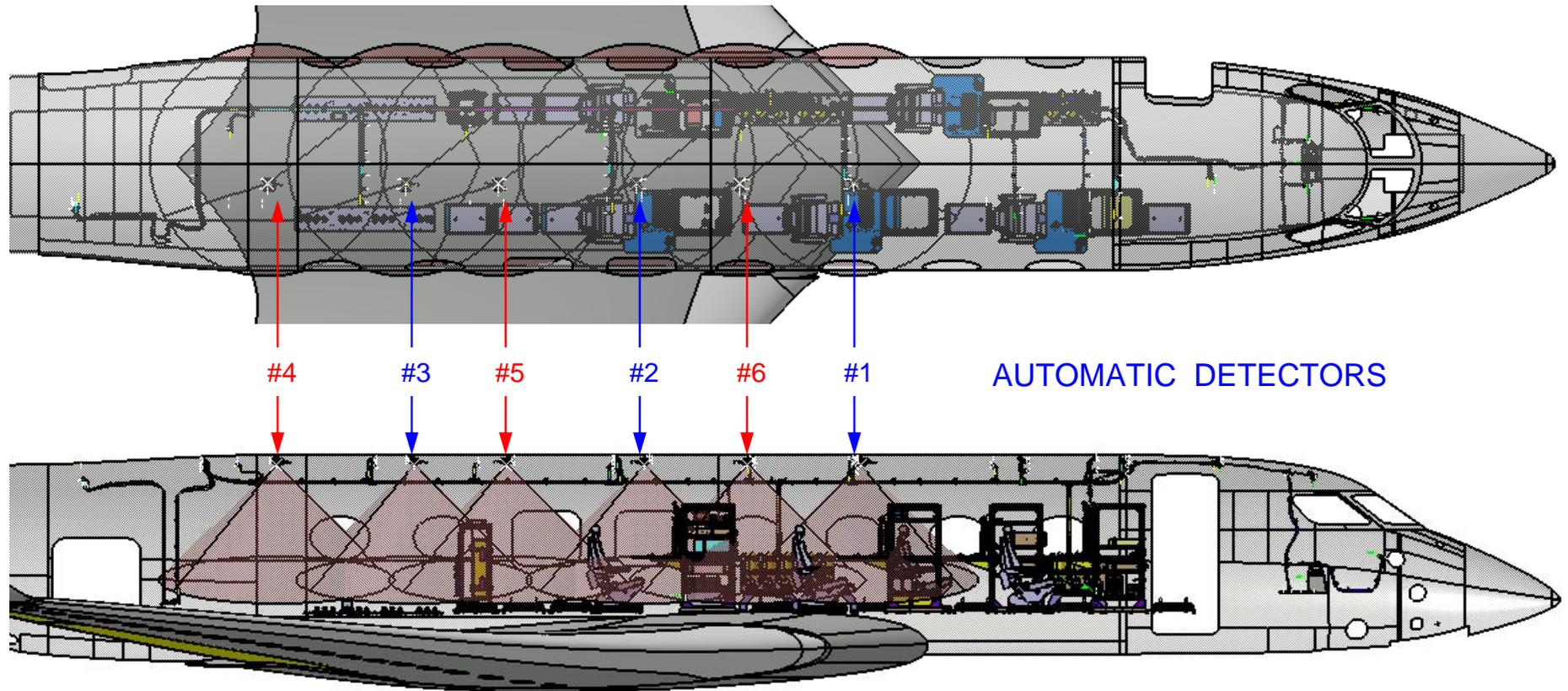
**3 sensors on each system for redundancy**
